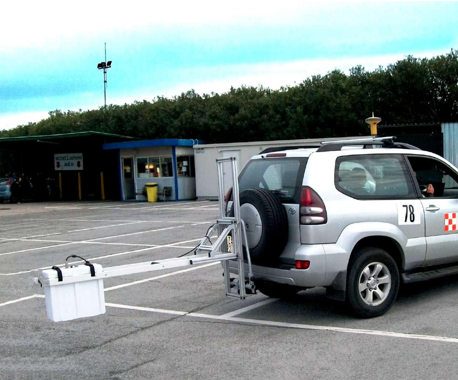
Providing a **complete assessment of road conditions** at unsurpassed speed with a **dedicated array of multi-frequency antennas**
