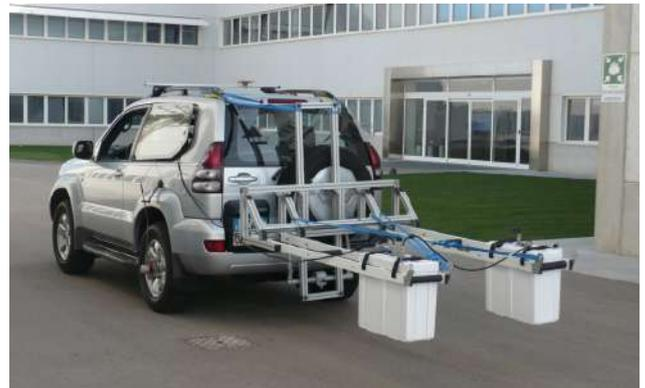
Dual horn antenna configuration
