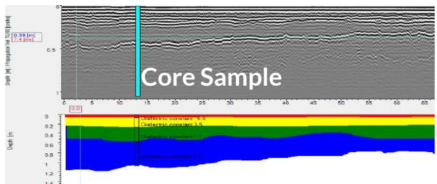
GRED HD 3D: post-processing software for subsurface layer extraction
