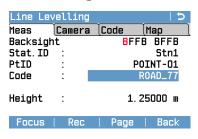
**Backsight/Foresight**: The selected levelling method. The current viewing direction is highlighted in red.
