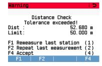
Example of warning message screen. The title of the screen describes which type of tolerance has been exceeded, e.g. the distance tolerance.
