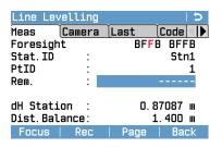
**dH Station**: Height difference on the current instrument station.
