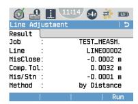
MisClose Comp.Tol Mis/Stn Method Calculated misclosure of the line at the second control point. Calculated closing tolerance according to the selected method.
