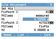
To reset the selected points and their heights to the default value, press **Reset**. To calculate the misclosure and to view the adjustment results, press **Cont**.
